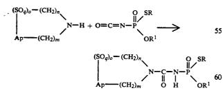
The reaction can be conducted by combining the two starting materials in a solvent, such as ether, toluene, methylene chloride, or acetonitrile at about  $-10^{\circ}$  C. to 65 about 60° C. and allowing them to react. The product, a compound of the present invention, that forms can be recovered by conventional means, such as by evapora-
