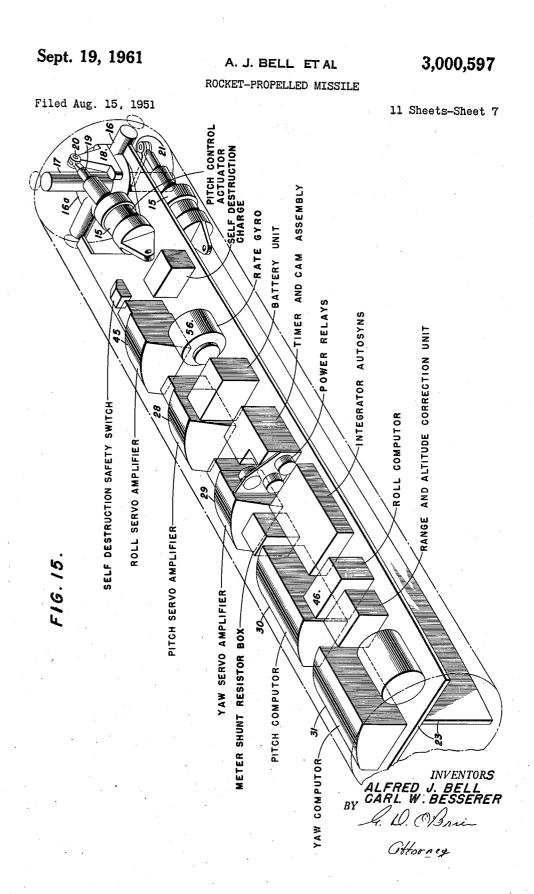
A. J. BELL ET AL ROCKET-PROPELLED MISSILE 3,000,597
