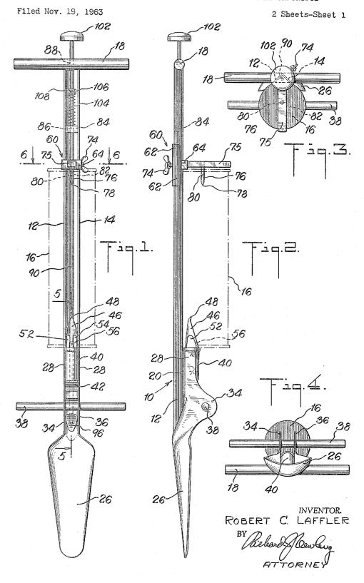
FERTILIZER DISTRIBUTING TOOL WITH REPLACEABLE CARTRIDGE
