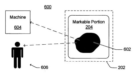
(57) Abstract: A marking beam (306, 212) of electromagnetic energy is generated within a printing device (102, 102') and a visibly markable portion (204) of a replaceable subsystem (202) that is at least partially arranged within the printing device (102, 102') is altered by illuminating at least part of the markable portion (204) with the marking beam (212).
