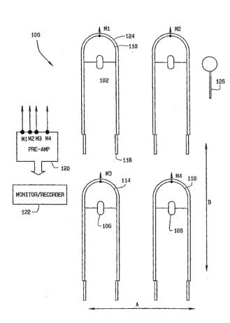
(57) Abstract: Method and apparatus comprising a method of recording natural sounds with a matched microphone array, recording the signal on a high resolution recording device including creating an audio bed, and playing back the recording on a tuned playback system. The method and apparatus is used to create or duplicate an ambient sound space for ambient therapy.
