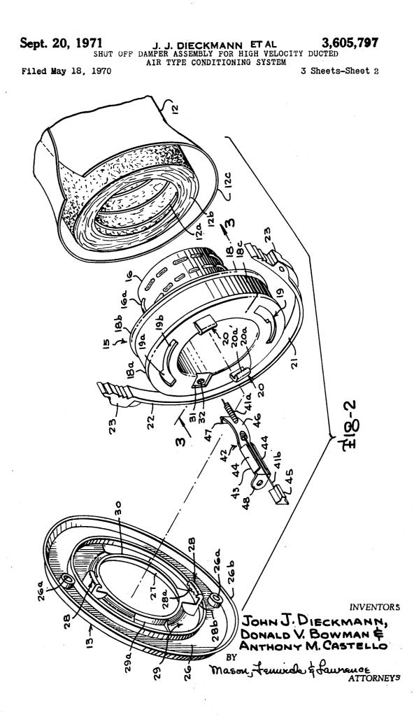
Sept. 20, 1971 SHUT OFF DAMPER ASSEMBLY FOR HIGH VELOCITY DUCTED AIR TYPE CONDITIONING SYSTEM Filed May 18, 1970 3 Sheets-Sheet 3
