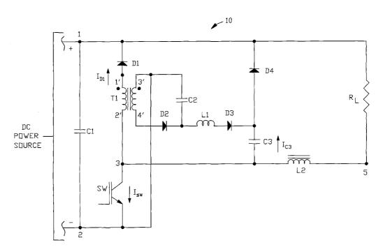
(57) Abstract: A solid state switching circuit utilizes a transformer in series with the circuit's switching device by which energy initially stored in the primary of the transformer is recovered in resonant circuitry connected to the secondary of the transformer for transfer of the energy to the load when the switching device is not conducting.
