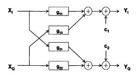
Figure 9 Analog Quadrature Modulator Compensation Block
