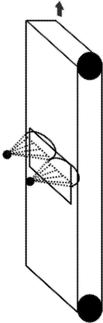
A) Moving Station with Multiple Spray Heads
