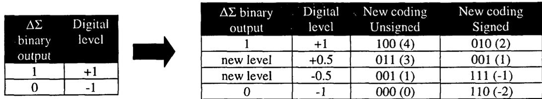
5 Schematics for these four recoding techniques are shown in FIG. 38A-D. Because of its simplicity and equivalent performance the unsigned insert zero technique is the preferred method of changing the dynamic receive delay in a digital  $\Delta\Sigma$  based beamformer. Also, due to the bit growth it is better to perform the delay change (slip) at the output of the delay line so that the extra bit does not need to be carried
