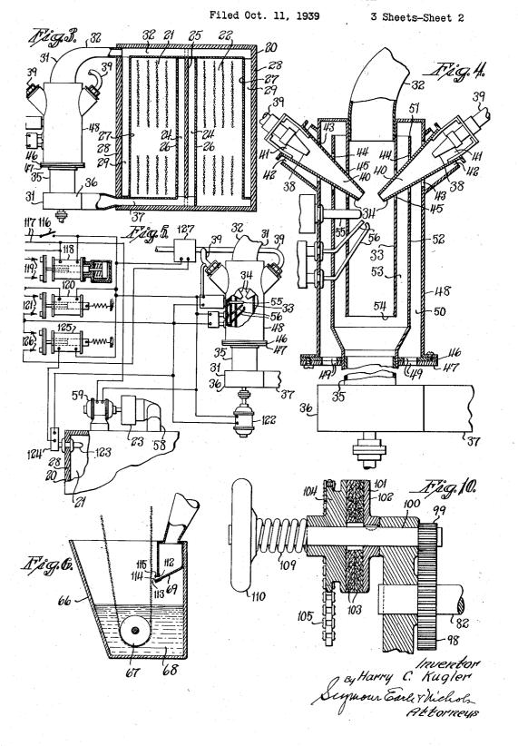
APPARATUS FOR DRYING WIRE SCREEN CLOTH
