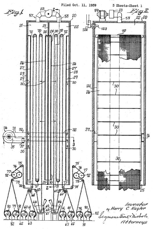
APPARATUS FOR DRYING WIRE SCREEN CLOTH
