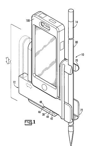
(57) Abstract: A method and device for holding an electronic device, such as a suitably-equipped cellular phone, having a video recording feature, or simply a camera, at a desired elevation for filming or photographing. The device includes a frame for holding the electronic device and a vertical support serving as a monopod, such as a golf alignment stick. The frame may be a two-part adjustable frame comprising two interlocking, opposing, L-shaped elements.
