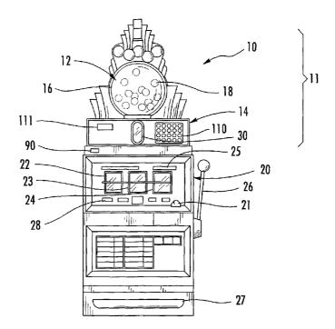
(57) Abstract: A gaming machine (10) includes a rotatable container (12) in which there are moveable objects (18). Upon activation of the rotatable container (12) the gaming machine simulates choosing a movable object (18) and displays a processor-selected object in window (30). The indicium on the processor-selected object may be used in a bonus game displayed in game matrix (110).
