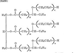
This compound is preferred due to its availability and to its ability to be purified to a high degree and thus the discoloration of the polycarbonamide to which it is added is extremely slight.
