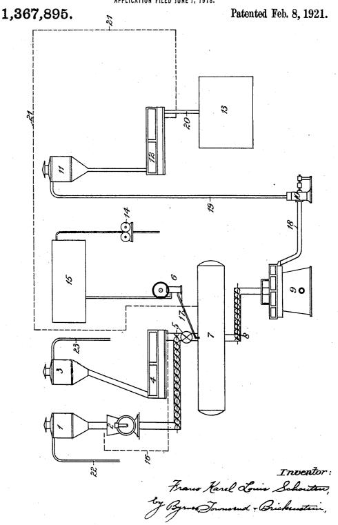
F. K. L. SCHOUTEN. PROCESS FOR THE MANUFACTURING OF FIBROUS MATERIAL FROM WOOD OR THE LIKE. APPLICATION FILED JUNE 1, 1918.
