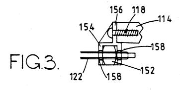
adjustment member and a screw-threaded region associated with the screw-threaded rod.
