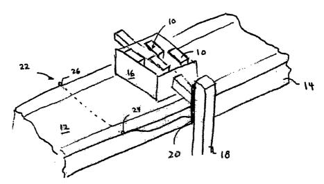
(57) Abstract: A printing apparatus comprises a jetting assembly (16) including a plurality of nozzles for ejecting droplets on a substrate moving relative to the jetting assembly, a mechanism for increasing the displacement of the jetting assembly relative to the substrate (20), and a sensor (22) configured to activate the mechanism for increasing the displacement of the jetting assembly upon detecting a predetermined dimension of the substrate surface relative to the jetting assembly.
