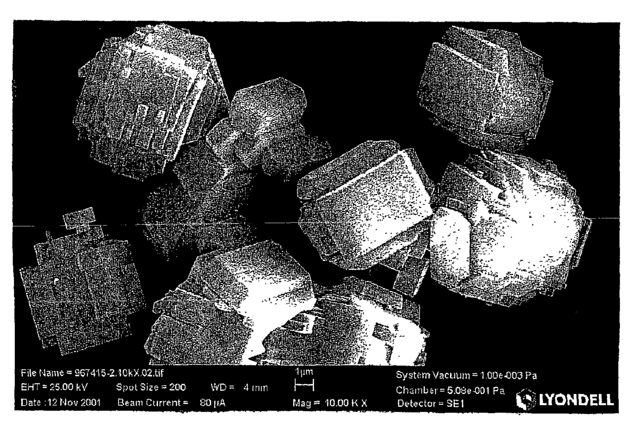
(57) Abstract: Large crystals of titanium silicalite or intergrowths of intergrown smaller crystals, having a mean particle size greater than 2 μm, have been found catalytically effective at commercially reasonable rates for the epoxidation of olefins in the presence of hydrogen peroxide. Crystals synthesized with a silica source having a low sodium content exhibit high levels of production and selectivity. The crystals have a low attrition rate and are easily filterable from a product stream.
