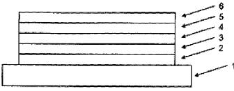
(57) Abstract: An organic optoelectronic device, such as an organic light emitting device, includes an anode (2), a cathode (4, 5, 6) and an active organic layer (3) between the anode and the cathode. The cathode includes a layer including a strontium compound (4), a first conductive layer (5) over the layer including a strontium compound, and a second conductive layer (6) over the first conductive layer, and provides a stable device.
