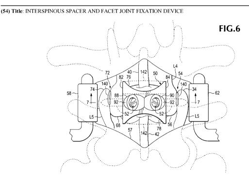
(57) Abstract: A biologically implantable device including a spacer body and fasteners for fixing the spacer body in place between vertebrae, and a method for use of the device to improve intervertebral spacing and correct foraminal stenosis, and to immobilize facet joints and promote fusion of adjacent vertebrae to each other. A drill guide may be used in providing bores in the facet joints to receive the fasteners.
