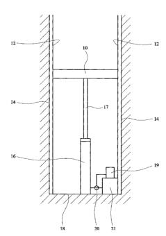
(57) Abstract: A hydraulically driven elevator or lift is provided with counterbalance means to at least partly counterbalance the load imposed by the load carrier or lift car. Operation of the counterbalance means, which includes a source of hydraulic fluid communicating with an accumulator, does not involve any interference with the working fluid of the hydraulic drive system.
