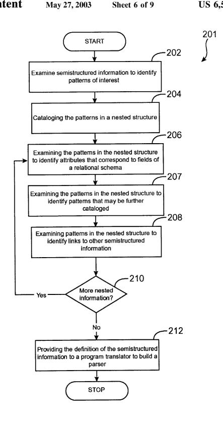
FIG. 2B (STEP 102 OF FIG. 2A)
