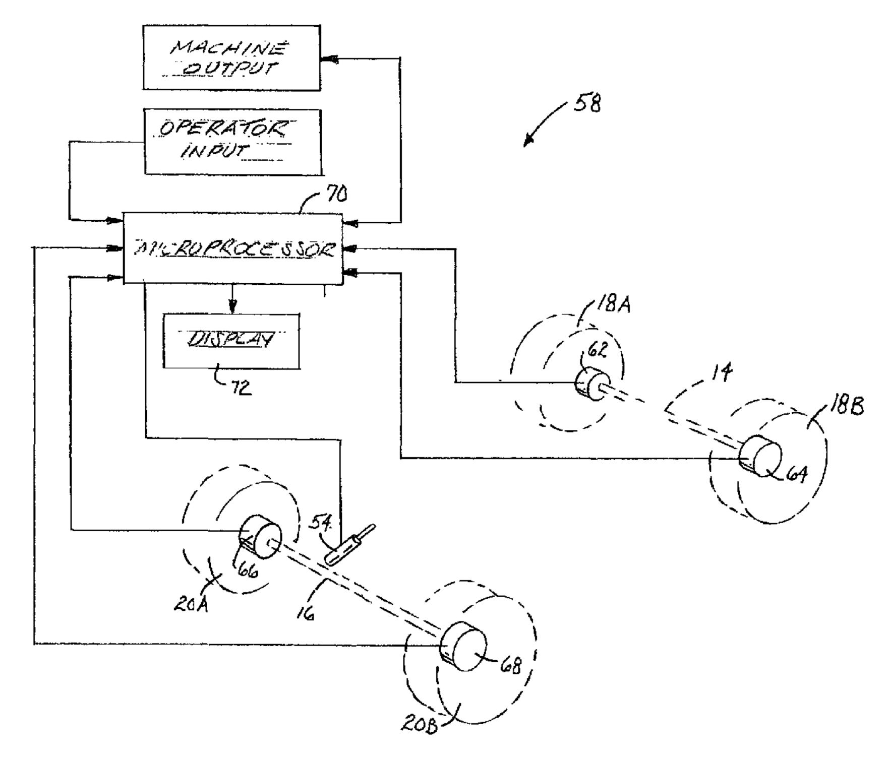
(57) Abstract: A material handler (10) that includes a frame (12), first and second front wheels (18A, 18B), first and second rear wheels (20A, 20B), and a control system (58). The front and rear wheels define a generally horizontal plane. The control system determines the center of gravity of the material handler and displays the location of the center of gravity of the material handlet within the plane.
