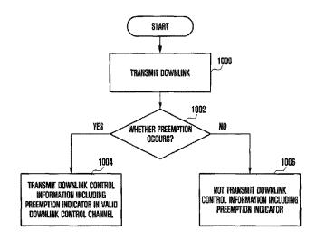
the second signal preempts the resource allocated to the first signal to the terminal when the second signal preempts the resource allocated to the first signal.
