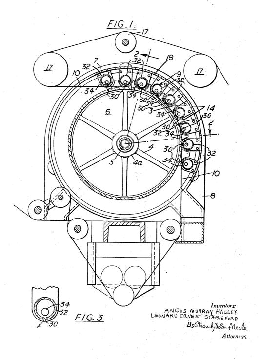
APPARATUS FOR DRYING PRINTED WEBS OF MATERIAL
