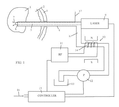
(57) Abstract: A system and method are described for ex-vivo, real-time NMR analysis of tissue removed either for purposes of biopsy or tissue removed during an ablation procedure.
