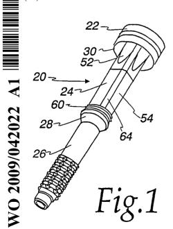
**(57) Abstract:** A milking machine teat cup liner having a dome and a barrel, and the barrel has an upper transition portion and a lower square portion. The transition section mates with the round cross-section of the dome and the square cross-section of the lower square portion to provide superior vacuum seal with less irritation and damage to teat tissue.
