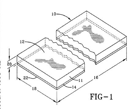
(57) Abstract: A construction board comprising a cellular body including at least one planar surface, where the cellular body includes a polyurethane or polyisocyanurate cellular structure, where the cellular structure has a density greater than about 2.5 pounds per cubic foot, an ISO index of at least 270, and where the cellular body includes at least 5.0% by weight flame retardant based on the weight of the cellular body.
