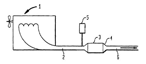
mixture of the supported vanadate component as a washcoat on the wall-flow filter or extruding a composition containing the supported vanadate component. The method of treating exhaust gases from an engine includes contacting the exhaust gas with the catalyst including the vanadate component.
