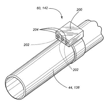
(57) Abstract: A hand cleaning tool (12, 134) for a floor cleaning apparatus includes a wand (44, 13, 138) and a light source (60, 42) that is carried on the wand and oriented thereto for directing light onto a surface being cleaned. A floor cleaning apparatus (10, 110) incorporating the hand cleaning tool is also described.
