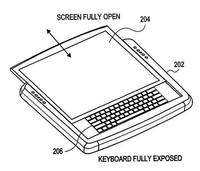
(57) Abstract: A mobile computing apparatus (202) that includes a sliding screen (204) and a keyboard (206) that moves from a storage position to a typing position in response to the screen being moved from a closed position to an open position.
