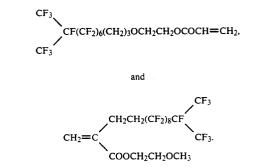
The block copolymer according to claim 1, wherein the residue M<sup>2</sup> is formed from a fluorine-containing monomer selected from the group consisting of:
