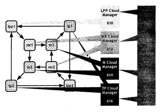
(57) **Abstract:** A distributed mediation network and method of employing such is provided, having a plurality of different types of network module. Each module has a non-reciprocal path therethrough for network traffic and the distribution of network traffic across the network is managed by an autonomic control plane.
