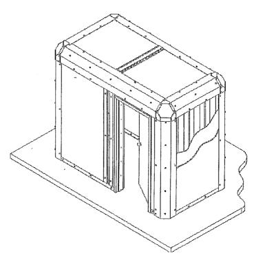
(57) Abstract: An assembly of wall panels particularly suitable for protection against wind blown debris or an explosion includes a bent strap connecting an air gap between adjacent wall panels with the bent strap capable of flexing due to a sudden external force.
