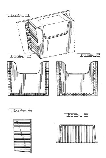
FIGURE 1 is a perspective view of a tissue package holder showing my new design;
