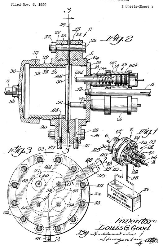
MULTI-RANGE FLUID FLOW MEASURING APPARATUS
