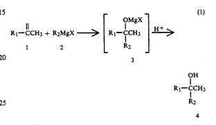
wherein R<sub>1</sub> and R<sub>2</sub> are alkyl groups such that the alkanol 4 is substantially straight chain and X is a halogen (e.g., chloro or bromo). The reaction is well documented in the art and involves reaction of ketone 1 with Grinard reagent 2 under suitable reaction conditions to provide for intermediate 3 which upon hydrolysis
