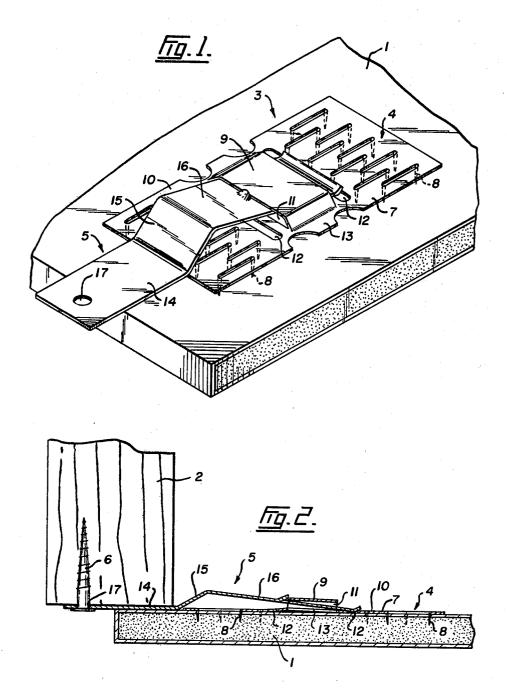
FASTENER FOR ATTACHING PANEL TO STUD
