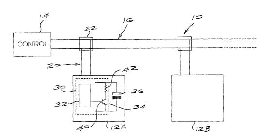
(57) Abstract: A detonator which, once armed, is automatically disarmed after a predetermined time period in the absence of at least one defined signal during such time period.
