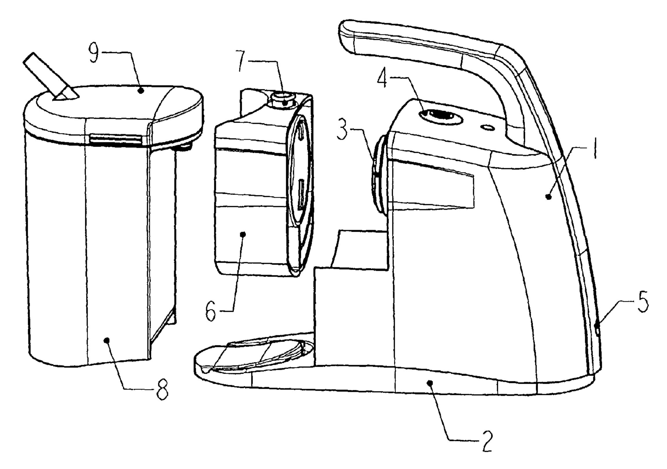
(57) **Abstract:** The inventive suction pump is essentially comprised of three separate pump parts, namely of a drive unit located inside a main casing (1), of a collecting reservoir (8) and of a valve block (6), which is arranged directly between the casing (1) and reservoir, whereby these parts can be easily coupled to one another in a manner that enables them to be detached.
