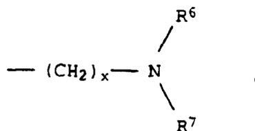
where R<sup>6</sup> and R<sup>7</sup> are identical or different, linear or branched C<sub>1</sub>- to C<sub>4</sub>-alkyl, or the two radicals together are C<sub>4</sub>- to C<sub>6</sub>-cycloalkylene, which may contain an -O- or -NR<sup>5</sup>- bridge in bonded form in place of a methylene group, and x is an integer of at least 3,
