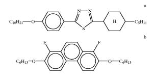
Liquid Crystal Mixture A: Phase transition temperature: Sc 64.3 Sa 77.2 N 81.4 I Ps:  $-8.2 \text{ nC/cm}^2$   $\Delta \epsilon$ : -2.7Tmin: 12  $\mu$ s Vmin: 23 V/ $\mu$ m 2 05V: 27.4°
