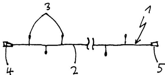
ing means (3) connected via an electric cable (2). A specific number of illuminating means (3) of an illuminating segment (1) is connected in series and the rows thus formed are connected in parallel.
