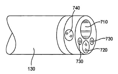
(57) Abstract: Delivery system including endoscopes are described. In an embodiment, a delivery system includes a flexible, elongate endoscope extending along a longitudinal axis when the endoscope is straightened and a first lens located on the distal region. The first lens faces a direction transverse to the longitudinal axis. The first lens permits the endoscope to provide an image of anatomical structures that offset from the axis of the endoscope.
