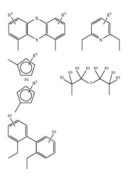
wherein X is selected from the group consisting of  $-O_{-}$ ,  $-S_{-}$ ,  $-Si(R^{a})_{2}$ ,  $-Si(OR^{a})_{2}$ ,  $-N(C(O)R^{a})_{-}$ ,  $-N(R^{b})_{-}$ ,  $-C(R^{c})$   $(R^{c})_{-}$ ,  $-C(O)_{-}$ ,  $-N(SiR^{d})_{-}$ ,  $-P(R^{d})_{-}$ , -P(O)  $(R^{d})_{-}$ ,  $-C=C(R^{c})$   $(R^{c})_{-}$  and  $-P(OR^{d})_{-}$ ,
