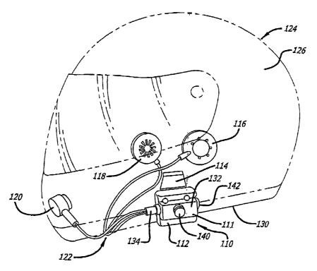
(57) Abstract: A communications system (110) is attached to a helmet (124,136) using a resilient clip (114) adapted to use spring forces to elastically and removably grasp the lower peripheral rim (130) of the helmet. Rigidly fixed to the resilient clip is a junction box (132). A microphone (120) and speakers (116,118) are attached to the helmet and are electrically connected to a transceiver through the junction box.
