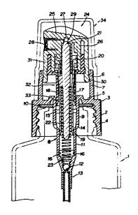
The present invention relates to an atomizer and, more especially, to a miniature atomizer of the manual type for atomizing a liquid such as perfume or a cosmetic preparation, the atomizer having a vertical reciprocating pump.
