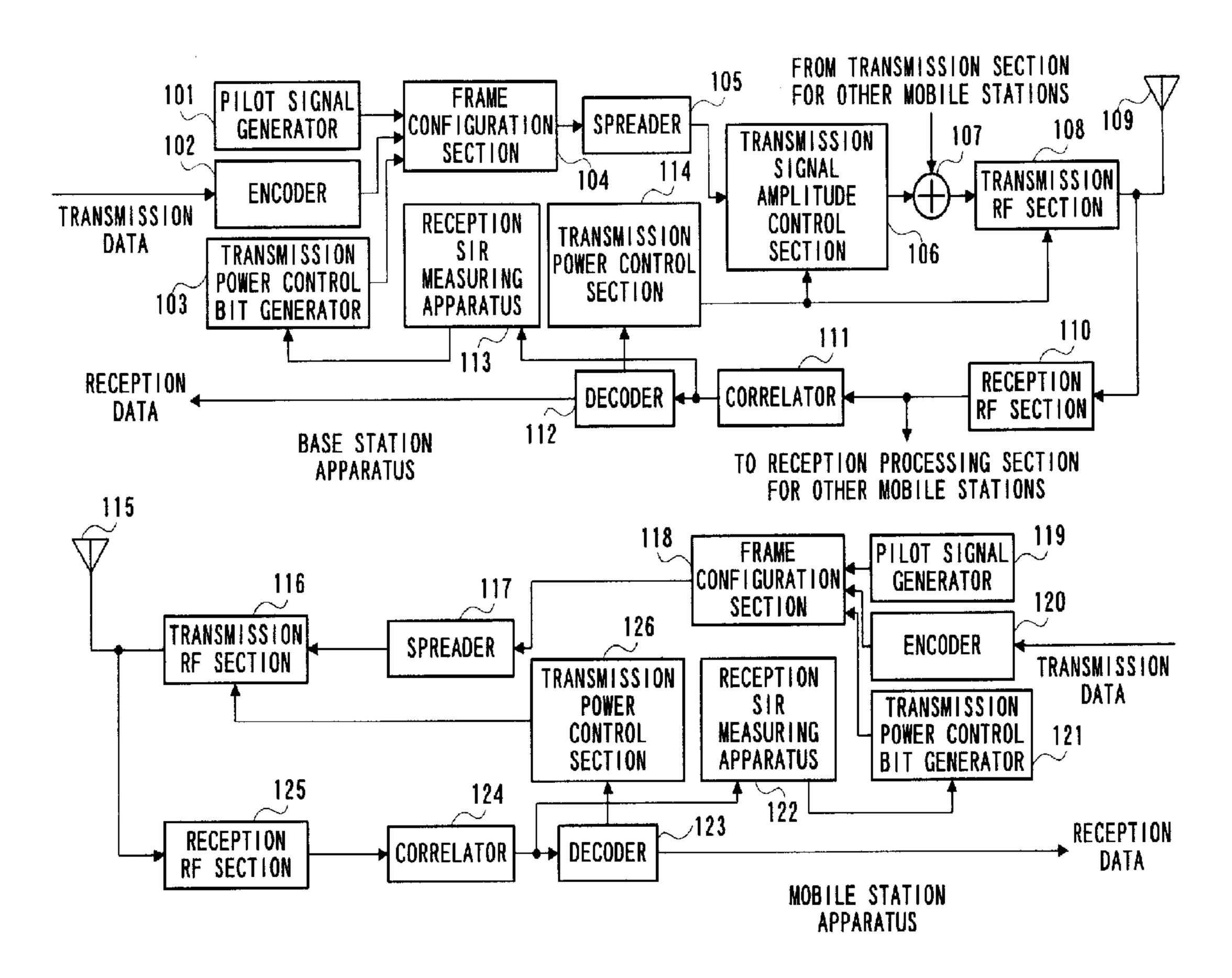
(57) The base station apparatus according to the present invention places pilot data and transmission power control data independently of each other in a slot based on processing delays and propagation delays required for transmission power control and places slots by providing an offset for the slot locational relationship between the uplink and downlink.
