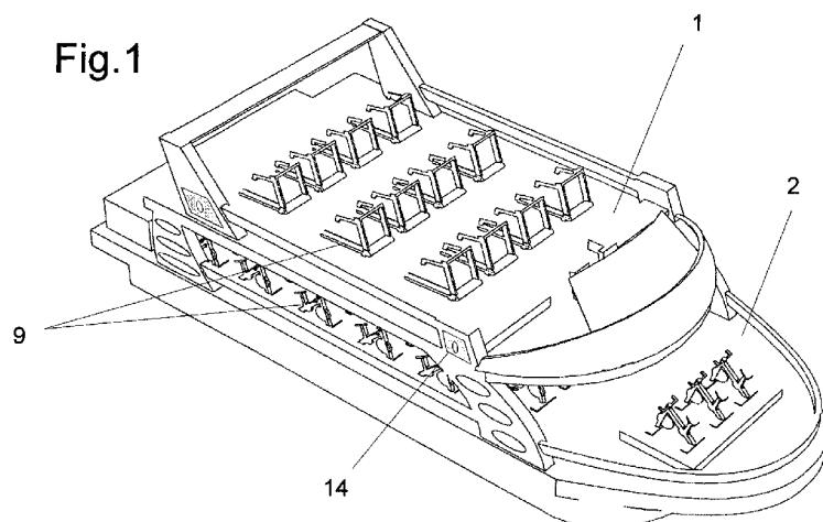
(57) Abstract : A barge with bicycles and treadmills installed in the deck thereof, and containing adapted energy generators that generate electric energy for recharging the batteries that power the propelling electric motors installed at the stern of the barge.
