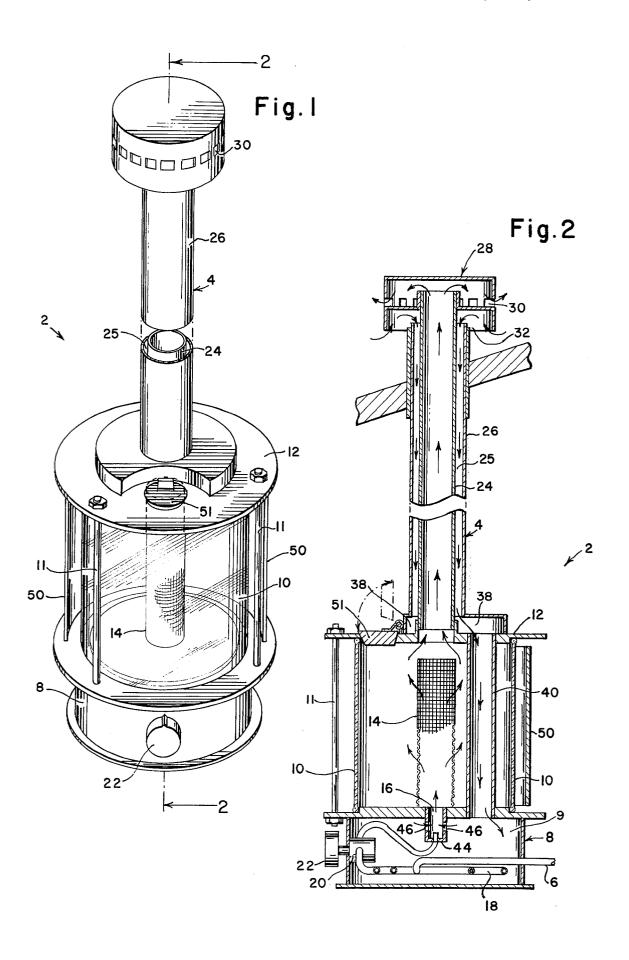
This invention relates to infrared space-heaters, and particularly to compact gas-fired heaters for uses such 5 as in recreational vehicles, boats and camping installa-
